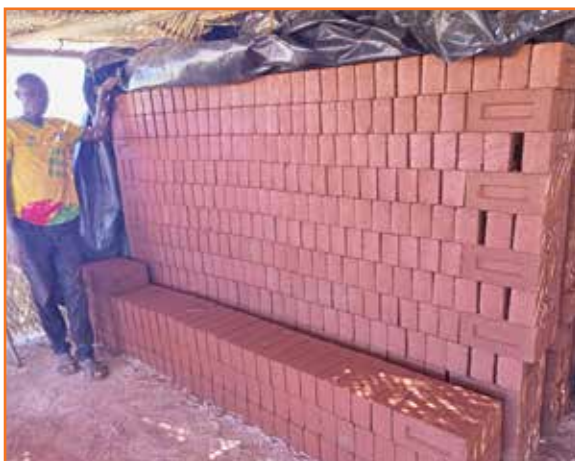
Earth bricks were made locally for the school construction
